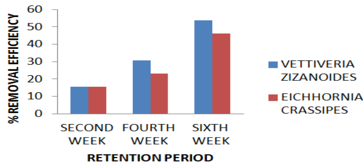
Figure 7: Effects of Ammonia in River Water by Hydroponic Plants for Different Retention Periods
