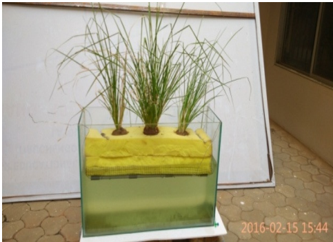
Figure 1: Installation of Artificial Floating Island
